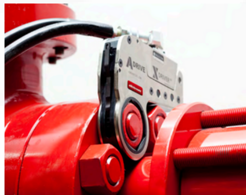
Application Example: A-Drive when fitting a flange coupling in plant construction.
